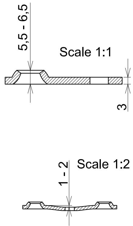
A little deformation in the flat holes areas is due to the working procedure.
